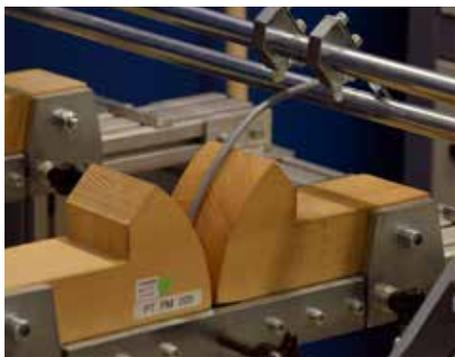
Flexural strength test
