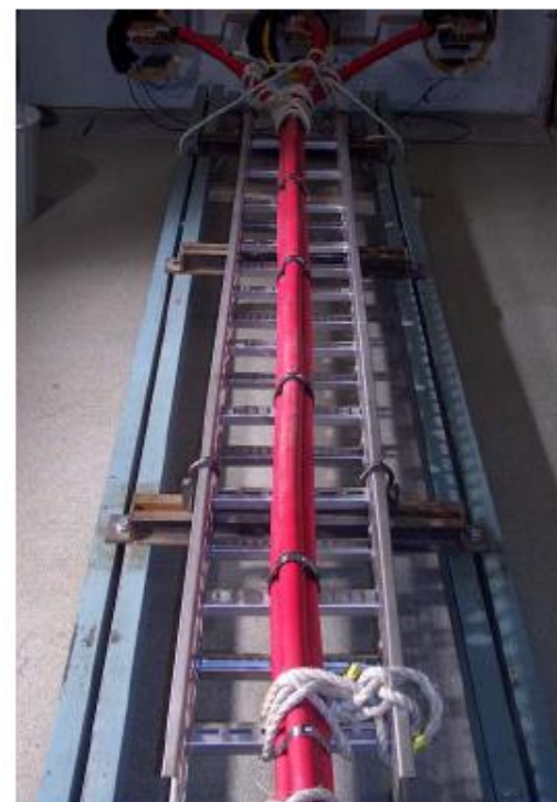
Figure 3: 240 mm 2 cable installation. Single loop cable ties with cushion sleeving mounted with a distance of 0,6 m.
