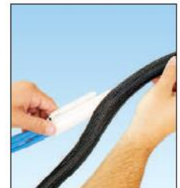
Grasp end of Pan-Wrap™ Braided Sleeving and bundle while pulling the tool along the bundle length.
